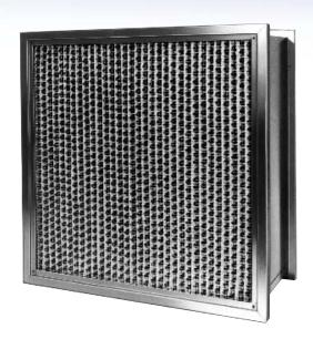
The advanced media in the DuraCel filter consists of minute glass fibers finely woven into a glass mat which is capable of withstanding temperatures up to 302°F/150°C.
