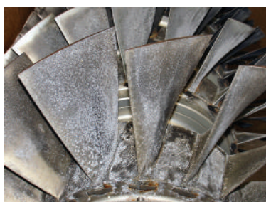
Titan 130 Compressor - 8,000 Hours with Frequent Water Washes
